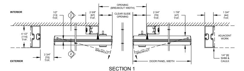
TYPE: P-SX-SX-P DOOR SHOWN IN OPEN POSITION WITHOUT THRESHOLD
