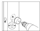
5.3.1 Drill a 2-1/8" [54] dia. hole on the door face from both sides to center of the door to avoid wood splitting.
