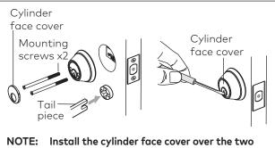
NOTE: Install the cylinder face cover over the two mounting screws.
