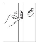
5.7.1 Postion the faceplate on the door edge and mark the two screw holes.
