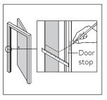
5.9.1 Locate and mark the center of the strike by measuring back from the door stop, 1/2" the thickness of the door.
