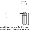
Additional screws for the door frame with 2 semi-round head screws is possible with SB.VAR.7 striking plate.
