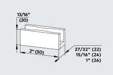
**RS 120 / RS 120 Syncro** floor guidea djustable **Ref. No. 907.126** Weight in lb (kg): 0.05 (0.024)
