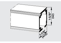
**RS track** Prepared for ceiling or wall mount, stock length 157" (4 m)
