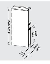
RS sidelite profile Connectable to track, non prepared, stock length 157" (4 m) Ref. No. 907.122 Weight in lb/ft (kg/m): 1.23 (1.680)
