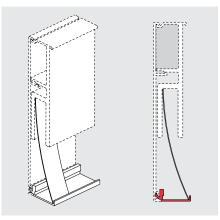
RS bottom view Protection profile (only in combination with sidelite profile 07.122 and cover profile 07.140) stock length 157" (4 m) Ref. No. 907.138 Weight in lb/ft (kg/m): 0.12 (0.164)
