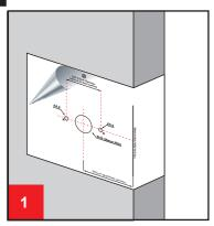
Position template and mark out drilling centres. Important also refer to lock/latch manufacturer's template prior to drilling. This template applies to bolt through fix lock/latch with a 60mm backset.
