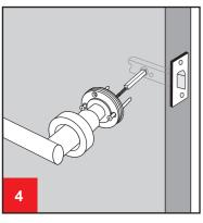
Insert spindle and spring supplied with levers to both sides of the door, as shown.
