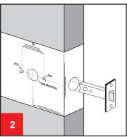
2. Drill holes in accordance with the template. Important Drill the 4.5mm holes half way through the door and repeat on the other side, with the holes meeting in the middle of the door.
