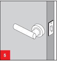
5. Install furniture to the door do not tighten screws with excessive tension on power driver as this may damage screws and void warranty. Screw on outer roses to lever set to complete installation.
