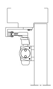
DOOR CLOSER MODELS: 7414, 7436 AO8P, AO10P PARALLEL ARM INSTALLATION (PUSH SIDE MOUNT)
