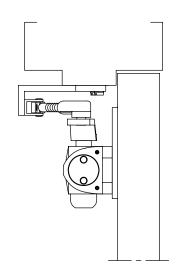
DOOR CLOSER MODELS: 7414, 7436 AO8P, AO10P PARALLEL ARM INSTALLATION (PUSH SIDE MOUNT) WITH PLATES DP74, DP86, DP86FC
