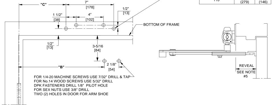
DOOR CLOSER MODELS: 7300 ISJ, ISJH TOP JAMB INSTALLATION (PUSH SIDE MOUNT) INTEGRA STOP ARM WITH PLATE DP73
