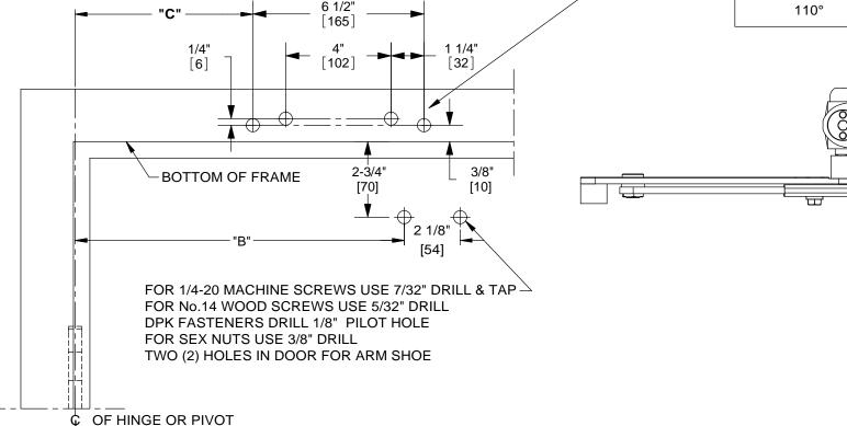
DOOR CLOSER MODELS: 7300 ISJ, ISJH TOP JAMB INSTALLATION (PUSH SIDE MOUNT) INTEGRA STOP ARM WITH PLATES BP73, BP86, BP86FC
