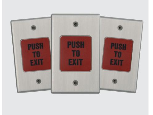
The RCI 917 easy touch is a pressure sensitive and solid state (no moving parts) switch. The square touch push button is weather-proof for a virtually infinite lifetime. The RCI 917 easy touch works with any system accepting momentary switch operation (SPST). The button is available with a handicap symbol or English, French, and Spanish "Push to Exit" labels.
