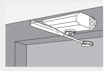
On the push side Transom fixing (Overhead installation)
