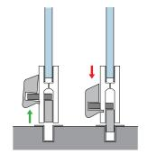
Door panel bolts are easily operated by simple activation with your foot.
