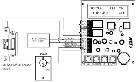
Note: FM Feature will only effect devices attached to Relay "A".
