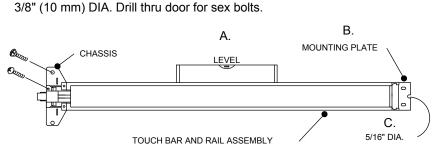
B. Fasten mounting plate (against rail) to door with (2) round head phillips screws.
