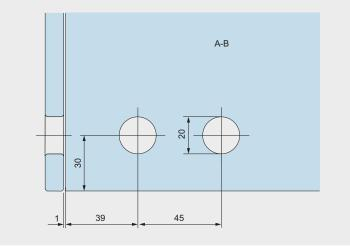
**PT 71** Overpanel connector with fin fitting 01.161
