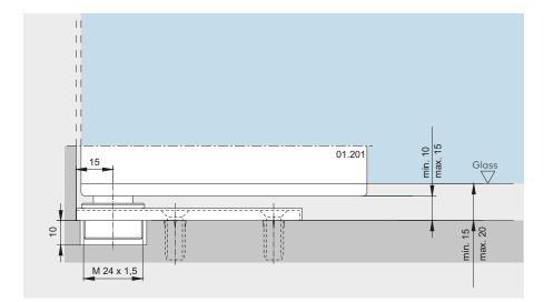
Using the bottom patch on pivot bearing with cover plate (Art. No. 01.201) the air gap between floor and glass is 15–20 mm (by height adjustability).
