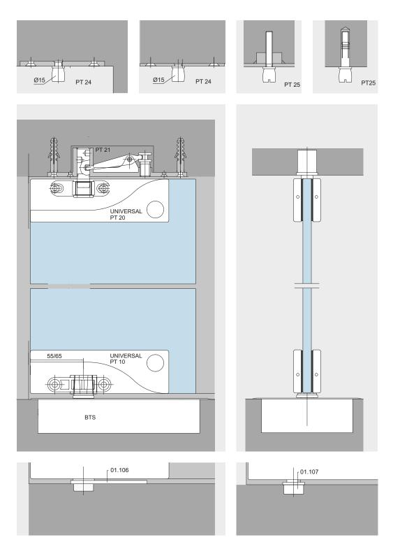
Fixing of top pivots and top centres for PT 20.
