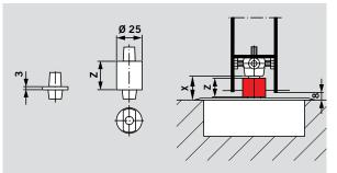
Calculating the necessary length of spindle extension: Extension =  $\mathbf{X}$  – Floor clearance (normally 8 mm) Collar height  $\mathbf{Z}$  of the extended spindle inserts = Spindle extension length + 3 mm (collar height of the standard spindle insert)
