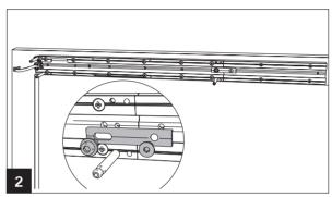
Drill two holes with a diameter of 5.5 mm into each of the outer grooves of the mounting plate extension.
