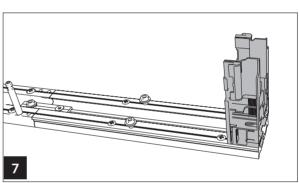
Slightly screw in the two thread-cutting screws for the bracket in the middle (a few turns will suffice).
