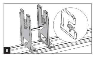
Lay the program switch cable in the groove and fix with clamping plates.
