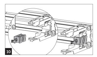
Wind up the remaining cables and fix them with cable ties to the centre bracket.
