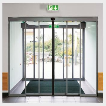
The TST FLEX Green telescopic sliding door is based on the same profile system as the ST FLEX Green sliding doors and is also an energy-saving sliding door specially designed for external building closure. The profiles have improved thermal separation and the thermal transmittance coefficients UD are proven by test certificates. Due to the slim profile elevations, this door type can be combined very well with the other door systems from the FLEX family.
