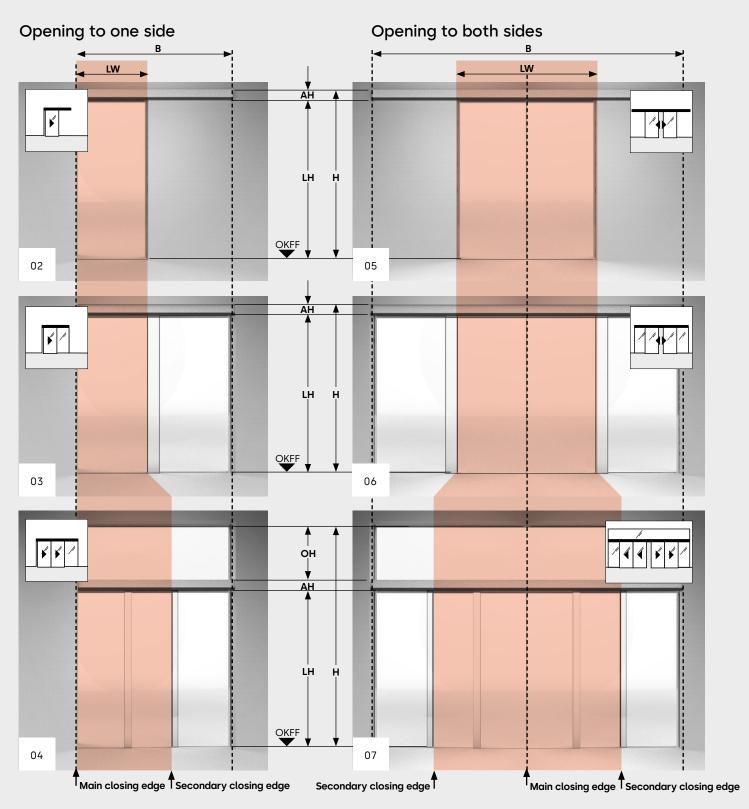
LW: Clearance width (passage width) LH: Clearance height (passage width)
