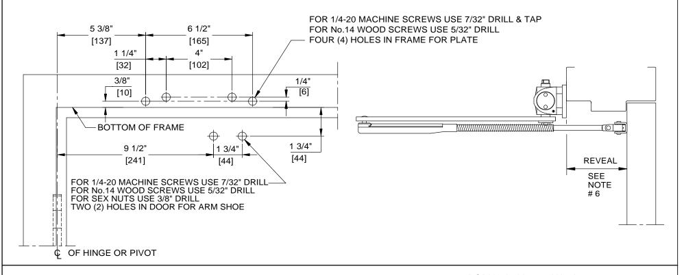
DOOR CLOSER MODELS: 7302 - 7305 ARNPJ (NHO) TOP JAMB INSTALLATION (PUSH SIDE MOUNT) WITH PLATES BP73, BP86, BP86FC
