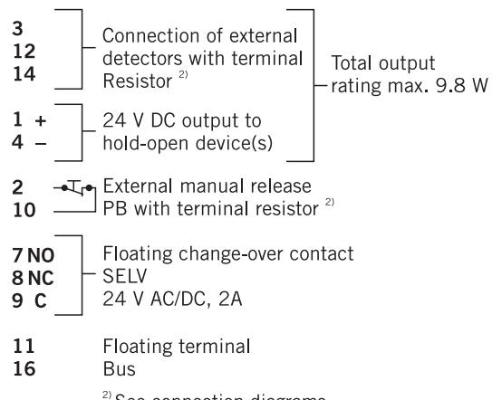
**4** Connect hold-open device(s) to terminals.
