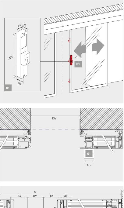
If the sliding door system is equipped with a manual release and a protective leaf, the clearance width LW is reduced by 83 mm for 1-leaf systems and 166 mm for 2-leaf door systems.
