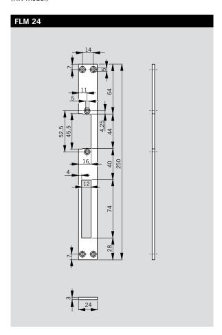
Flat strike plate of stainless steel, non-handed, for combination with DORMA electric strikes, Series Smoke, Fire 447 and Fire 442.
