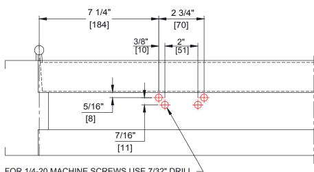
FOR 1/4-20 MACHINE SCREWS USE 7/32" DRILL OF No.14 WOOD SCREWS USE 5/32" DRILL DPK FASTENERS DRILL 1/8" PILOT HOLE FOUR (4) HOLES IN FRAME FOR PA BRACKET
