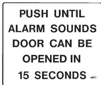
Several building codes including the NFPA 101 Life Safety Code and the International Building Code require the signage (shown left) to be mounted on each door close to the releasing device.
