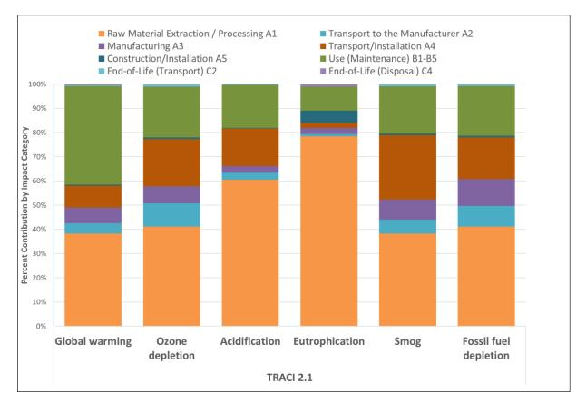
Figure 2. Contribution analysis for the Skyfold products - TRACI 2.1. (excluding product replacements).
