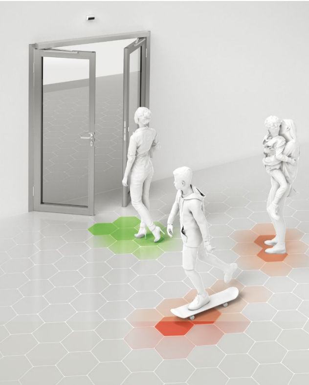
Short hold-open time with fast passage. Door closes immediately after the person has passed through.
