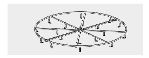
Floor element with stainless steel plate for sealing, measure X = 150 or larger
