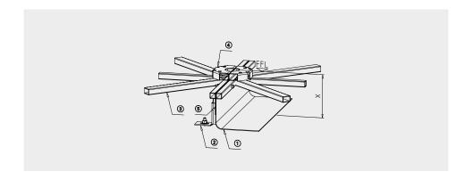
Floor element with drive box for floor pit, measure X = 350 or larger
