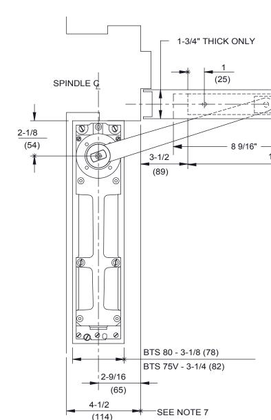
FOR WOOD SCREWS PROVIDED USE 5/32" DRILL TWO (2) HOLES IN DOOR
