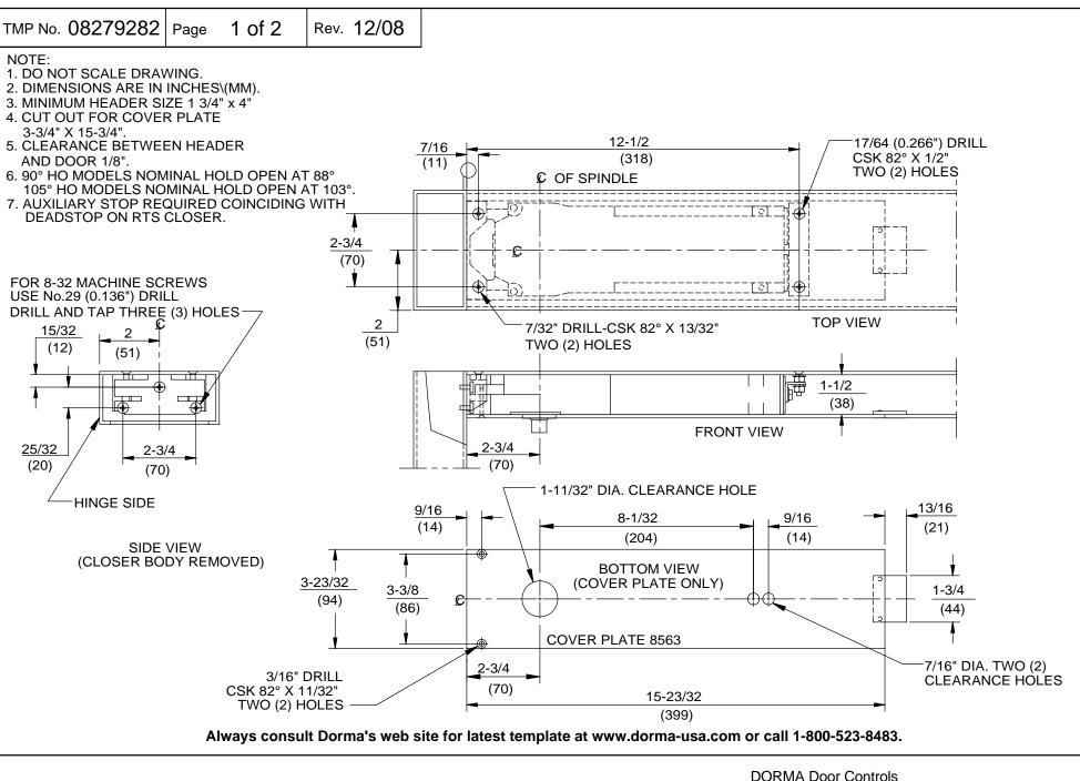
DOOR CLOSER MODEL: RTS SERIES PACKAGE 30, WOOD DOOR AND ALUMINUM FRAME PREPARATION, No. 8812 TRACK ARM, No. 8563 COVER PLATE, DOOR HUNG ON 4-1/2" WIDE BUTT HINGES
