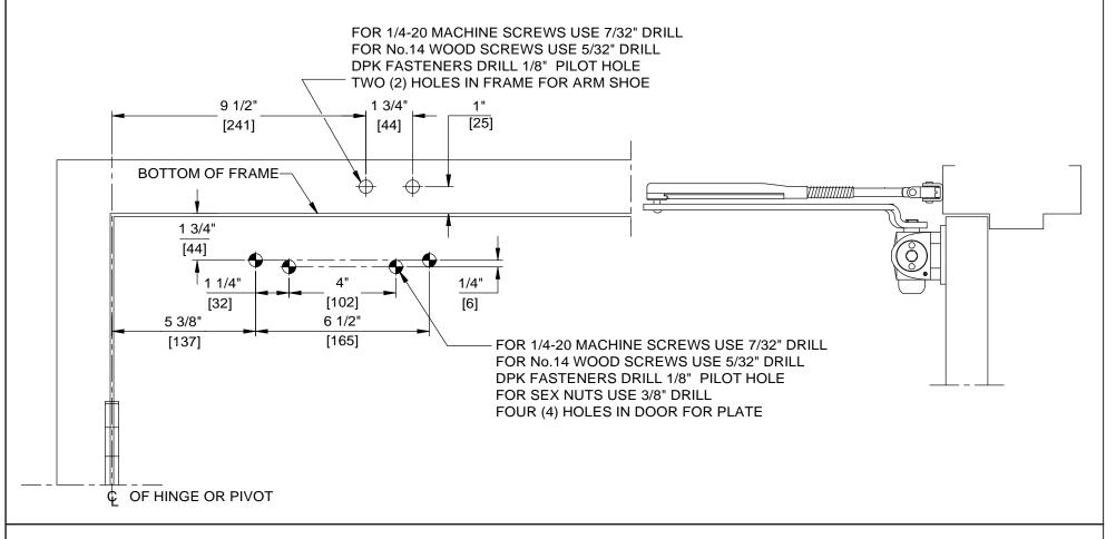
DOOR CLOSER MODELS: 7414, 7436 AR (NHO) REGULAR INSTALLATION (PULL SIDE MOUNT) WITH PLATES BP74, BP86, BP86FC
