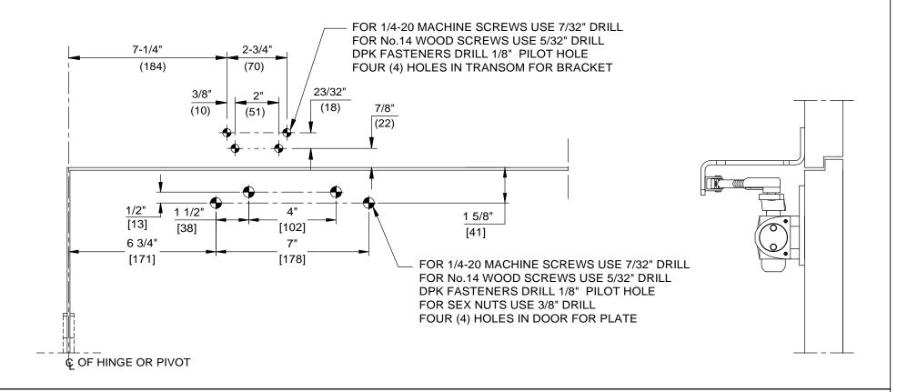
DOOR CLOSER MODELS: 7414, 7436 AR x PFT (NHO) PARALLEL ARM FLUSH TRANSOM INSTALLATION (PUSH SIDE MOUNT) WITH PLATES DP74, DP86, DP86FC
