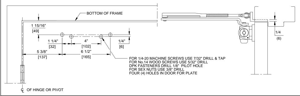
DOOR CLOSER MODELS: 8616 AR, AF x MJ REGULAR INSTALLATION (PULL SIDE MOUNT) WITH PLATES BP86, BP86FC
