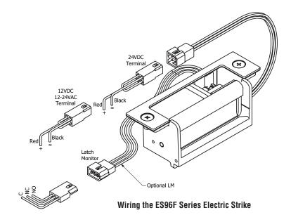
Model ES96F must be connected to a compatible UL Listed Access Control Power Supply.
