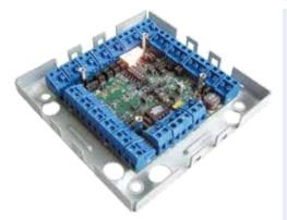
reader connections supporting multiple door modes, such as single door secured exit or two individual doors using a "Request for Exit" configuration.
