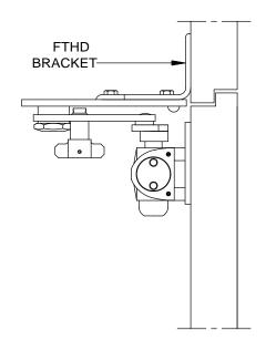
DOOR CLOSER MODELS: 8616 SPA, SPAT, SPAK, x FTHD SUPER PARALLEL ARM FLUSH TRANSOM INSTALLATION (PUSH SIDE MOUNT) WITH PLATES DP86, DP86FC
