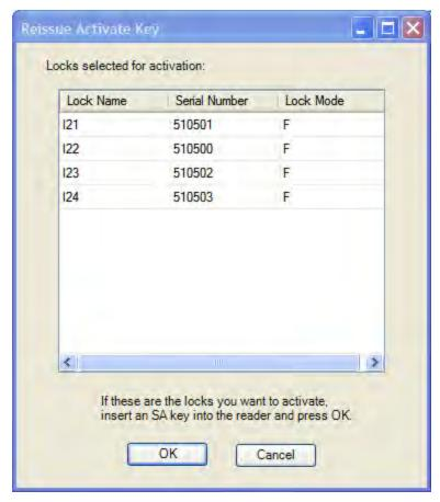
If the list is correct, insert an SA key into the reader and press OK. The message "SA Key Reissued" is displayed when the key is ready.
