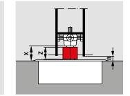
Calculating the necessary length of spindle extension: Extension = X – Floor clearance (normally 8 mm)
