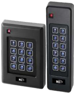
CSR-6.2L CSR-6.4L (mullion) 13.56MHz Smartcard & BLE Keypad Reader Ideal for dual authentication or simple access via PIN or credential applications. CSR-6.2L: 1.78" W x 6.1" H x 0.91" D (45 x 155 x 23 mm) CSR-6.4L: 3" W x 4.6" H x 0.75" D (76 x 117 x 19 mm)
