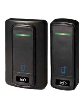
PCR-35L 125kHz & BLE Reader Unique design accommodates single gang or mullion mounts. Functions with 125 kHz physical and mobile (BLE) credentials Mullion: 1.7" W x 4.7" H x 1.2" D (43 x 119 x 30 mm) Switch Plate: 3" W x 5.1" H x 1.2" D (76 x 130 x 30 mm)
