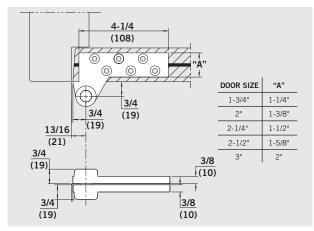
**No. 75140** — 3/4" offset brass top pivot for lead-lined doors 1-3/4" thick.
