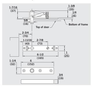
**HD8062** — Heavy-duty walking beam top pivot with frame portion and cover plate. Door portion consists of a needle bearing pressed into a 3/4" thick aluminum block. Adjustable to obtain a 1/8"–3/8" clearance between the door and frame. Required when using overhead stops/holders.
