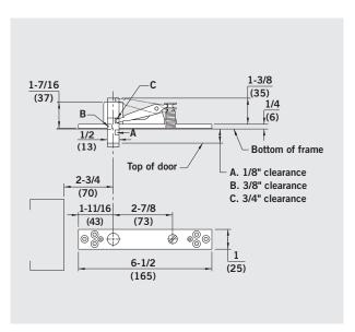
**8062.5** — Walking beam top pivot frame portion with cover plate. Pin has a 1/2" diameter.
