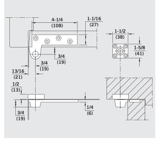
**No. 75120/102** — Standard mortised door portion with a pivot block containing a needle bearing mortised into the overhead condition above. This pivot is ideal for conditions when the door is inset from the frame face, or the ceiling is directly above the door.
