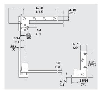
**No. 75320** — 3/4" offset brass bottom side jamb pivot. For use with doors weighing up to 350 lb. Has a vertical height adjustment of 3/8".
