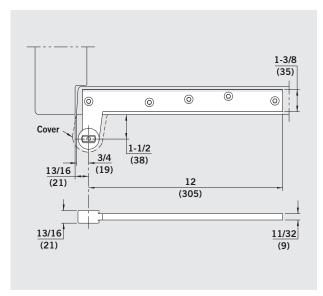
No. 15323 — 1-1/2" offset standard steel bottom arm. Can also be used on fire doors rated up to 3 hours. For use with 7471K and 7471HD floor bearing.
