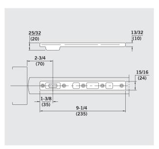
**No. 7421** — Center hung bottom arm for steel or wood doors. For use with 7471K and 7471HD floor bearing.
