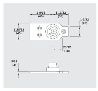
No. 7471K — Standard floor bearing with thrust roller bearing for doors weighing up to 440 lb. Can also be used on fire doors rated up to 3 hours. Includes cover cap. Mounts directly to floor. For use with No. 75323, 75343, 7421, 7422 and 15323 bottom arms. Available with integral spindle extensions as shown in the adjacent chart.
