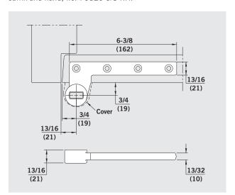
**No. 75323** — 3/4" offset standard steel bottom arm. Can also be used on fire doors rated up to three hours. For use with 7471K and 7471HD floor bearing. **(Specify Hand)**
