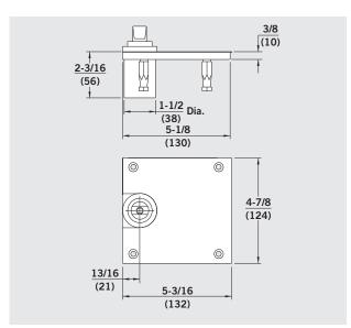
No. 7471HD — Heavy-duty floor bearing for center hung doors weighing up to 1000 lb and offset hung doors weighing up to 800 lb. Can also be used on fire doors rated up to 3 hours. For use with No. 7421, 75323, 75343 and 15323 bottom arms. Interchangeable spindles provide for bottom door clearances of 3/8" to 1-3/4". Includes cover plate. Bearing is mortised into floor. Interchangeable spindles and associated bottom door clearances shown in the adjacent chart.
