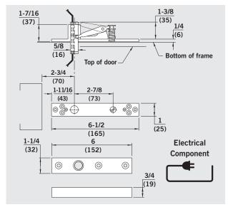
**E8062** — Electrified walking beam top pivot for power transfer. Available in a two wire and four wire design using #18 AWG. Both designs provide a maximum of 6 A at 24 V. Specify number of wires required.
