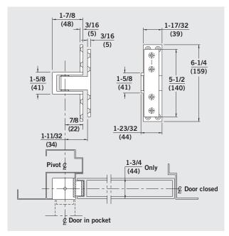
No. 75520 — Bronze pocket pivot. For 90° pocket doors. No. 75523 — Steel pocket pivot for 90° pocket doors, U.L. listed for 20 minute wood doors and 3 hour rated steel fire doors.
