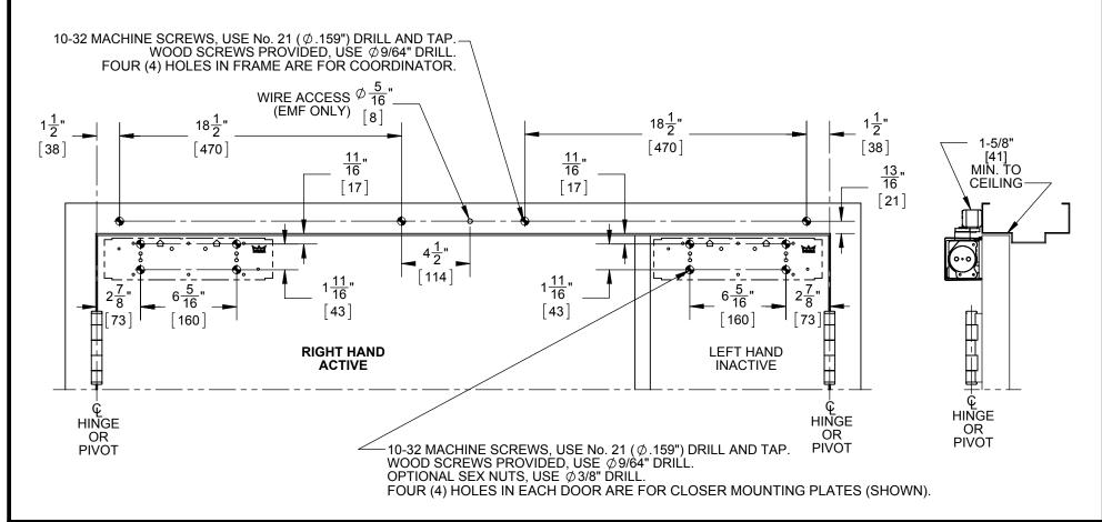
DOOR CLOSER MODELS: TS93 GSR/T, GSR/T EMF 1A, 1I TRACK INSTALLATION (PULL SIDE MOUNT) WITH DOOR COORDINATOR FOR 12" INACTIVE LEAF
