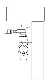
DOOR CLOSER MODELS: 7200/7300 A08P PARALLEL ARM INSTALLATION (PUSH SIDE MOUNT)
