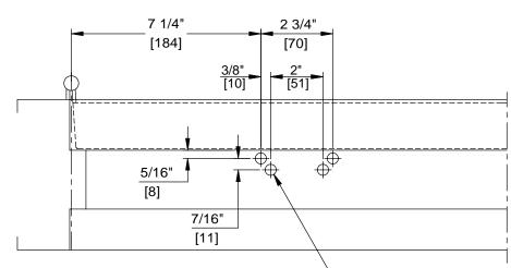
FOR 1/4-20 MACHINE SCREWS USE 7/32" DRILL FOR No.14 WOOD SCREWS USE 5/32" DRILL DPK FASTENERS DRILL 1/8" PILOT HOLE FOUR (4) HOLES IN FRAME FOR PA BRACKET
