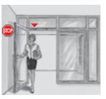
The mechanical hold-open device enables doors to be held without fallback at an opening angle up to approx. 120°.
