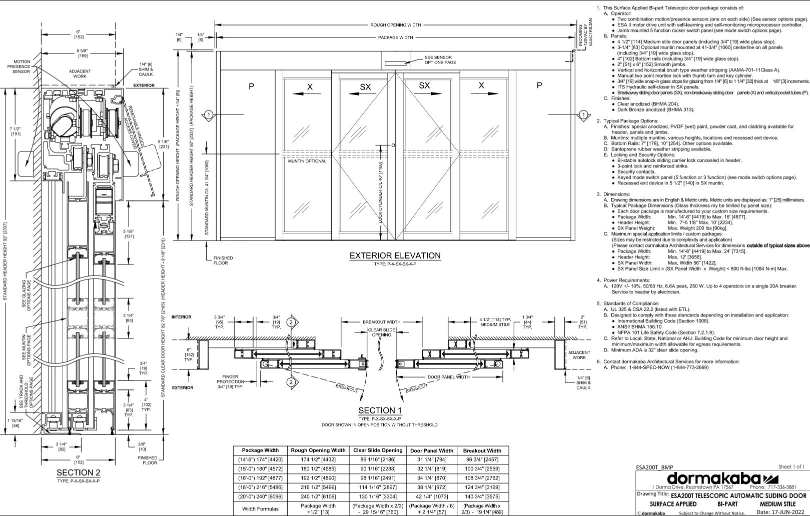
1. This Surface Applied Bi-part Telescopic door package consists of:
