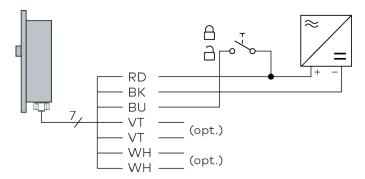
When in Fail Secure configuration, applying positive voltage to the control wire triggers the SL30SGL to unlock (active-low locking signal). In the event of a power cut, the SL30SGL will remain locked.
