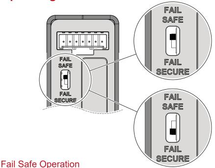
Assume the lock is installed, wired, and set to fail safe. The door is open and the positive supply voltage is applied to the **BLUE** wire. As the door closes the SL30SGL senses the door approaching and activates the bolt pin to pull the door into alignment. The Bolt Position and Door Position monitors will have changed to closed contact state as the door is closed and secured.
