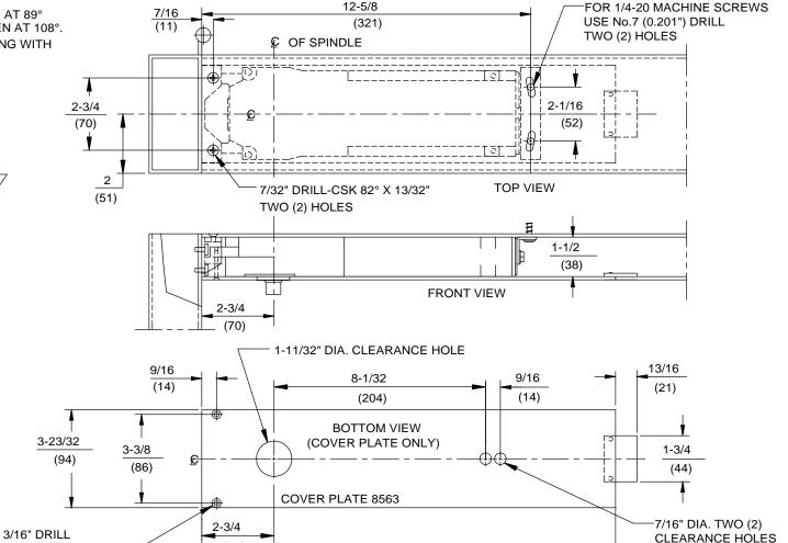
DOOR CLOSER MODEL: RTS SERIES PACKAGE 25, ALUMINUM DOOR AND FRAME PREPARATION, DOOR HUNG ON 4-1/2" WIDE BUTT HINGES, No. 8812 TRACK ARM, No. 8563 COVER PLATE WITH SLOTTED ANGLE BRACKET
