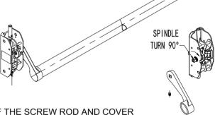
6) CUT THE LENGTH OF THE SCREW ROD AND COVER ACCORDING TO BELLOW LENGTH REQUIREMENT...
