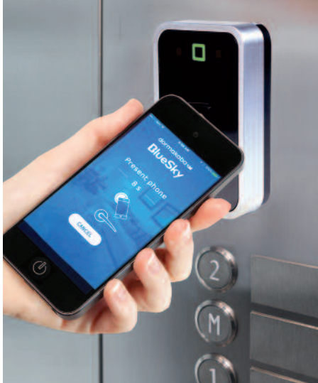
RAC5 elevator floor control
