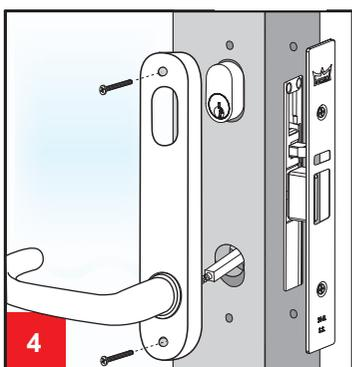
4. Insert spindle and spring supplied with lever to both sides of the door (spring locates fully into lever). Determine the correct screw length to suit the door thickness then cut screws.
