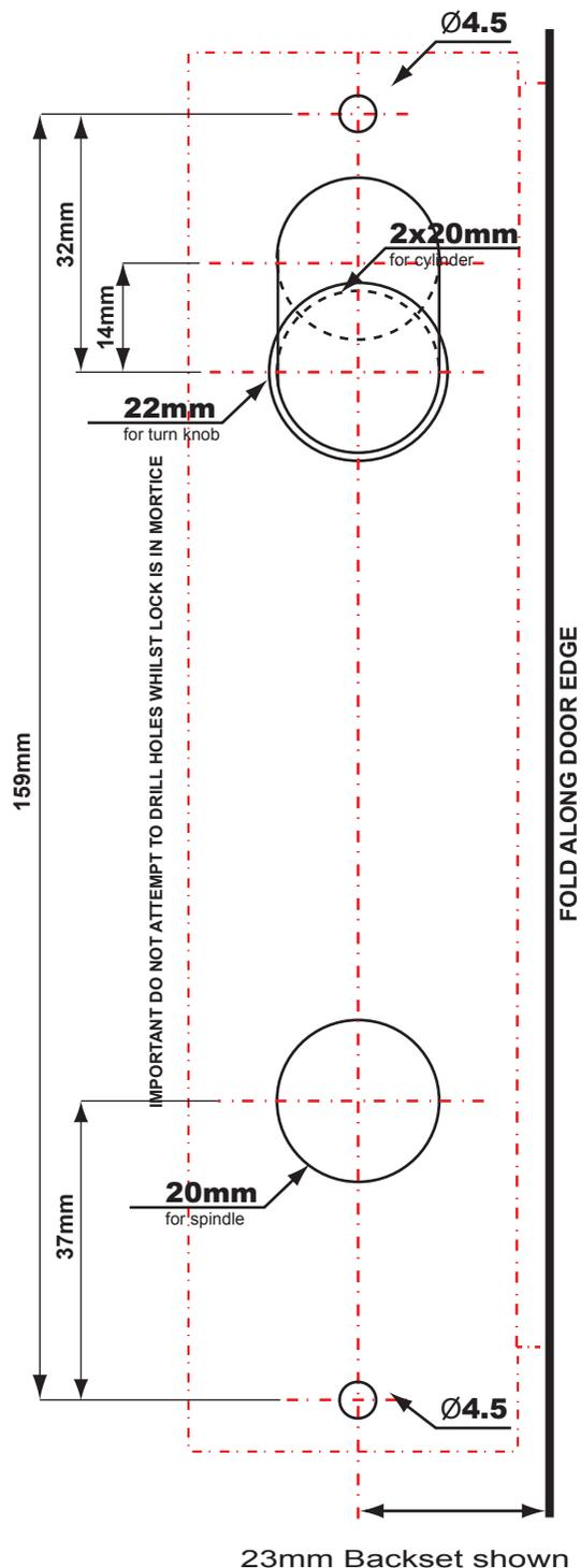
Paper templates might distort due to air moisture. Only the indicated measurements are therefore obligatory.
