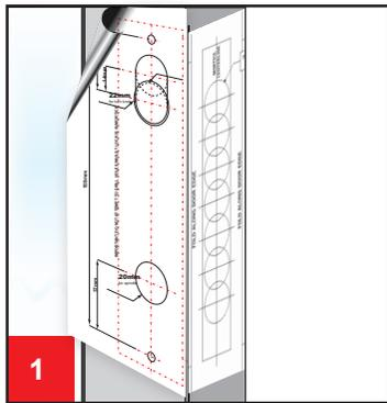
1. This template applies to bolt through fix lock/latch with a 23mm backset. Position template and mark out drilling centres. **Important** also refer to lock manufacturer's template prior to drilling.
