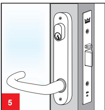
5. Install furniture to the door. Do not over tighten screws with excessive tension on power driver as this may damage screws and void warranty.
