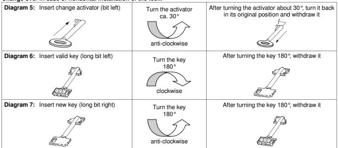
Change over in case of horizontal installation of the lock:
