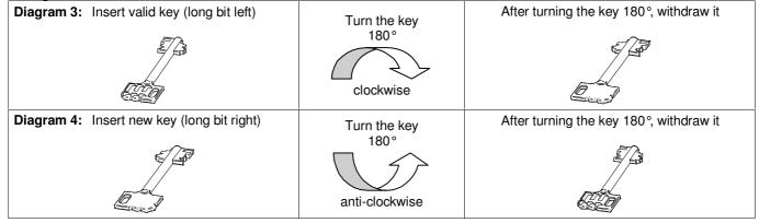
In case of vertical installation of the lock, the insert and withdraw positions of the keys change accordingly.
