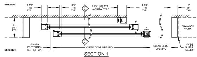
TYPE: P-X-X SHOWN, X-X-P OPPOSITE DOOR SHOWN IN OPEN POSITION WITHOUT THRESHOLD
