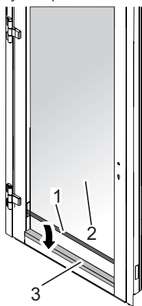
Fig. 37: Mounting the glass clamping profile
