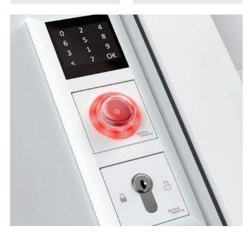
The SCU-UP with emergency button is always used with a key switch (e.g. analogue ST 55 key switch). Together with an electrical locking device, the SCU-UP fulfils the requirements of EN 13637 and EltVTR (German directive for electrical locking systems on escape route doors).
