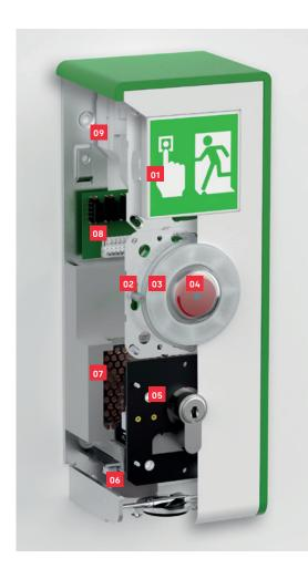
The STL-G door terminal is comprised of an emergency button and key switch in a surface-mount casing. Together with an electrical locking device, the STL-G door terminal fulfils the requirements of EN 13637 and EltVTR (German directive for electrical locking systems on escape route doors).
