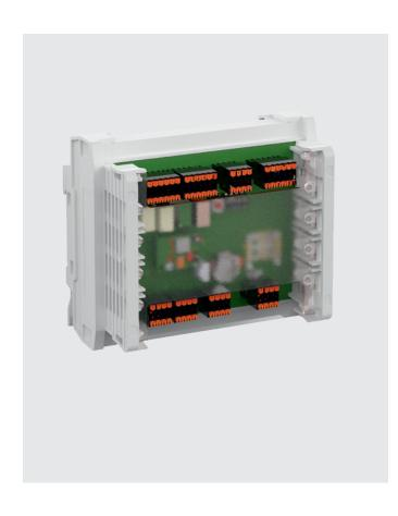
Together with a licence card, the SCU-DR is operated as a control and monitoring panel (master). For setting up an emergency exit and escape route system in accordance with BS EN 13637 or EltVTR, at least one emergency button and one key switch (e.g. SCU-UP 2-item supply set or STL-G surface-mounted terminal) as well as a rod lock door locking device are necessary. Mounting is done on a DIN rail or in the NT G1 / NT G2 housing.
